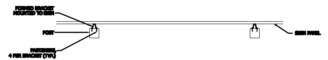
1 SIGN PANEL ATTACHMENT DETAIL SCALE: NOT TO SCALE
