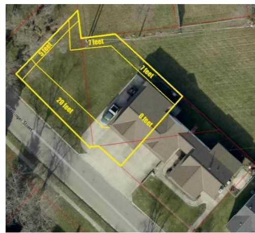
Proposed setbacks for zero-lot line development utilizing garage (consistent with P&Z approval in 2021).
