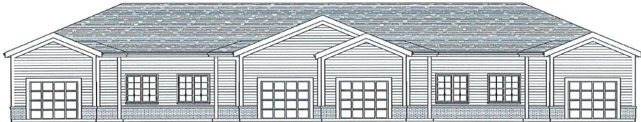
② Front 1/8" = 1'-0" Total Surface Area: 1,655.46 sf Surface Area - Excluding Openings: 1,231.72 sf Area of Brick: 172.46 sf Brick to Total Surface Area: 10.42% Brick to Surface Area Excluding Openings: 14.00%
