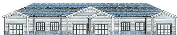
① Front 1/8" = 1'-0" Total Surface Area: 1,585.02 sq ft Surface Area - Excluding Overhangs: 1,271.12 sq ft Area of Sides: 272.25 sq ft Area of Roof: 30.65 sq ft Total to Surface Area Excluding Overhangs: 15.87%
