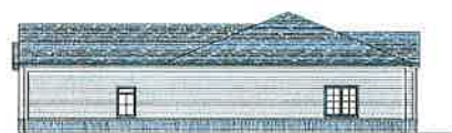
② Right Side 1/8" = 1'-0" Total Surface Area: 788.75 sq ft Surface Area - Excluding Overhangs: 714.38 sq ft Area of Sides: 64.37 sq ft Area of Roof: 9.00 sq ft Total to Surface Area Excluding Overhangs: 8.17%
