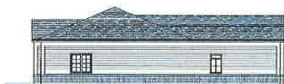
④ Left Side 1/8" = 1'-0" Total Surface Area: 788.75 sq ft Surface Area - Excluding Overhangs: 714.38 sq ft Area of Sides: 64.37 sq ft Area of Roof: 9.00 sq ft Total to Surface Area Excluding Overhangs: 8.17%
